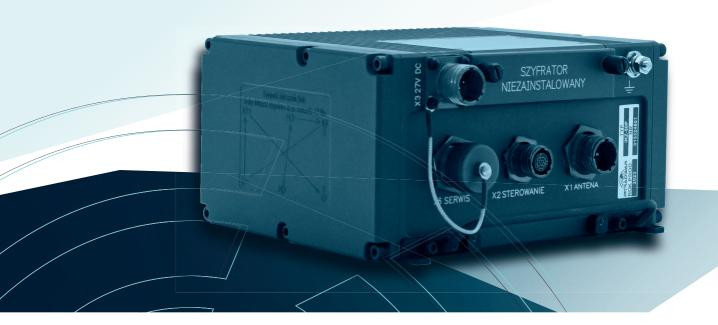
The IKZ-50P is a short-range IFF Mark XIIA interrogator designed for close-range air defense systems (SHORAD and VSHORAD) and is specifically tailored for integration with weapon systems and radars. It supports both fixed and rotating antenna platforms, ensuring flexible deployment.
