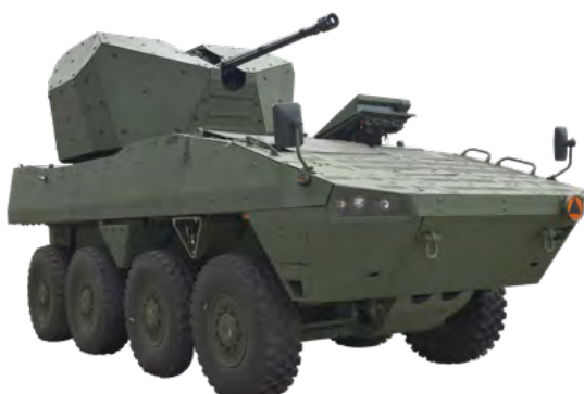
35 mm automatic gun system on the Rosomak vehicle
