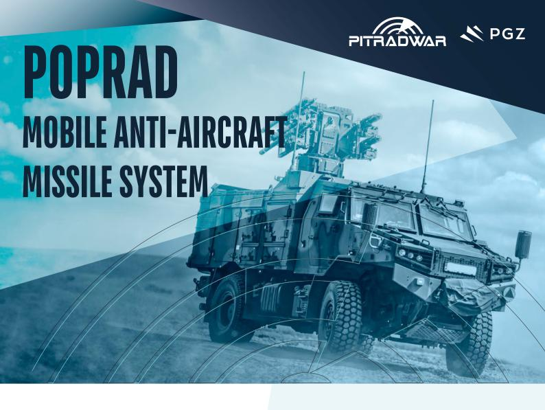
The POPRAD Self-propelled Anti-Aircraft Missile System (SPZR POPRAD) is intended for detection, identification and engagement short-range and low altitude air targets with the use of self-guided short-range missiles (heat-seeking missiles). The SPZR POPRAD might be used to cover columns of troops, staging points, command posts and military troops, as well as airports, harbors, industrial plants, communication hubs, etc. from air-strike means.
