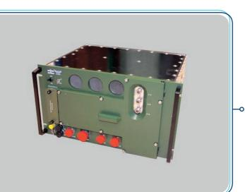
The interrogator has a flexible interfacing of the identification result usage (optical indication, voice messages, including range to interrogated contact, by serial RS422 port) and a flexible interfacing of the interrogation control (wire control, remote control, by serial RS422 port, remote control, by radio link).
