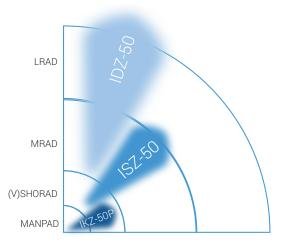
The IDZ-50 is a long-range interrogator dedicated for use with large-area surveillance radar and LRAD systems. The device's high output power and capacity make it a perfect complement to long-range primary radar systems.
